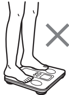
Your feet are not correctly positioned on the electrodes.
